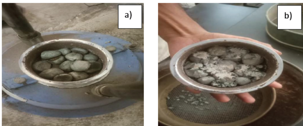
Figure 4: Aggregate impact testing a) the sample before and b) after test.
